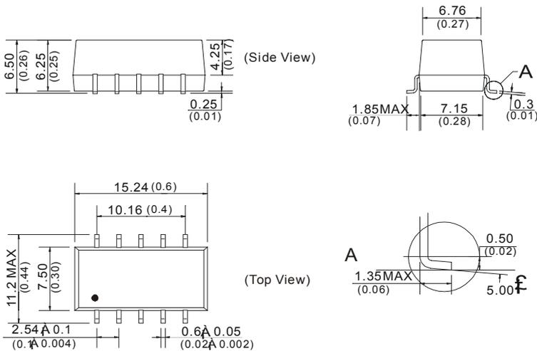
Note: All Pins on a 2.54mm(0.1) pitch; All Pin Widths are 0.60 mm(0.02); Tolerances: ±0.15mm(0.006); Unit: mm(inch)
