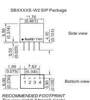
Top view,grid:2.54mm(0.1inch) diameter:1.00mm(0.039inch)
