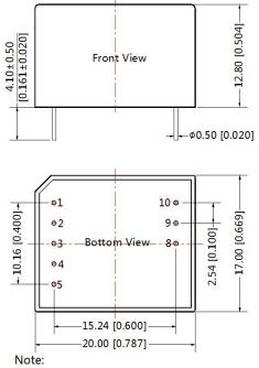
Unit :mm[inch] Pin diameter tolerances :±0.10[±0.004] General tolerances:±0.25[±0.010]
