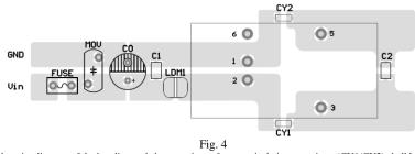
Note: the min. distance of the bonding pads between input & output isolation capacitors (CY1/CY2) shall be  $\geq$  2mm.
