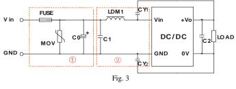
Notes: Part 1 in the Fig. 3 is used for EMS test and part 2 for EMI filtering; selected based on needs.
