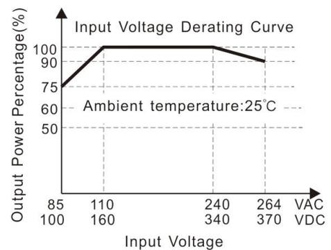
Note: ① With an AC input between 85-110V/240-264VAC and a DC input between 100-160V/340-370VDC, the output power must be derated as per temperature derating curves;
