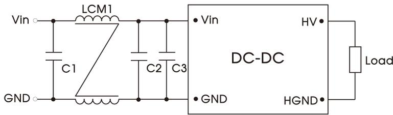
Fig.2 EMC recommended circuit
