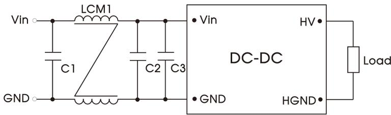
Fig.2 EMC recommended circuit
