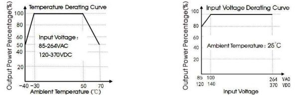
Note: 1) With an AC input between 85-100VAC and a DC input between 120-140VDC, the output power must be derated as per temperature derating curves; 2) This product is suitable for applications using natural air cooling; for applications in closed environment please consult factory or one of our FAE.
