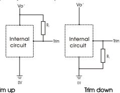
TRIM resistor connection (dashed line shows internal resistor network)
