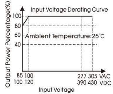
Note: ① With an AC input between 85-100V/ a DC input between 100-120VDC, the output power must be derated as per temperature derating curves;
