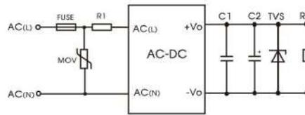
Fig 2: EMC application circuit with higher requirements
